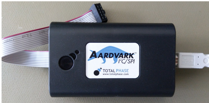
Figure 9: Aardvark bus to USB adapter
